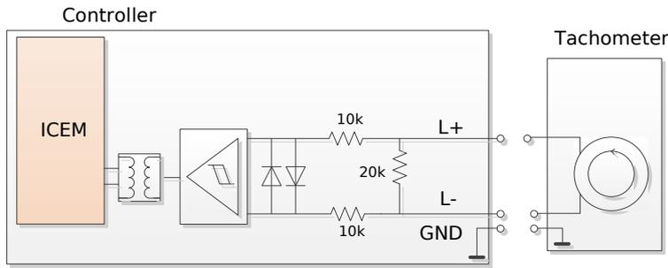
Picture 8 Connection of IC engine tachometer
