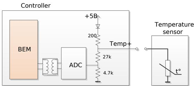
Picture 9 Connection of resistive temperature sensor
