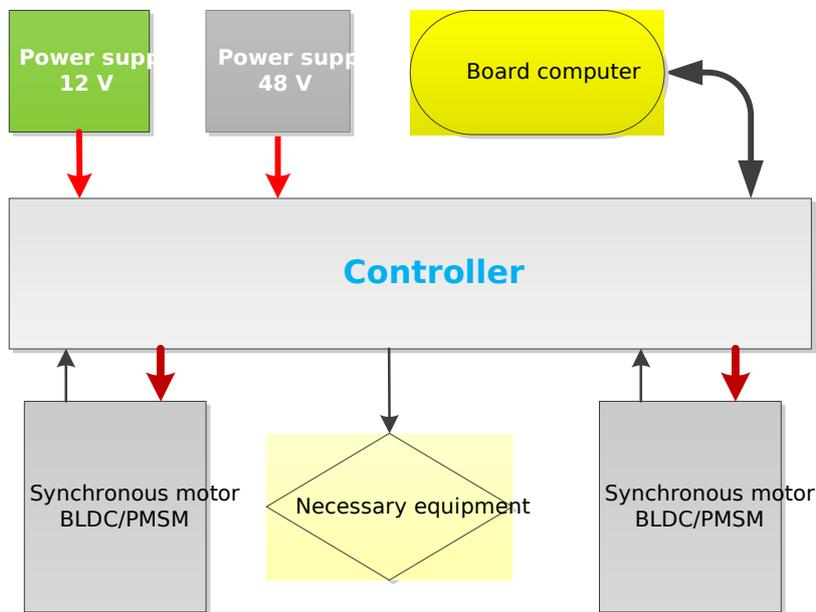
Pic. 19 Application of controller for the minimal configuration
