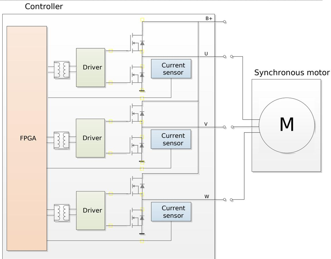
Picture 4 Synchronous motors connection
