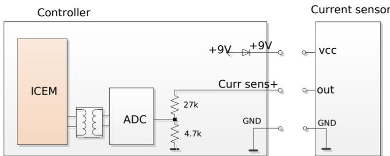
Picture 12 Connection of generator current sensor
