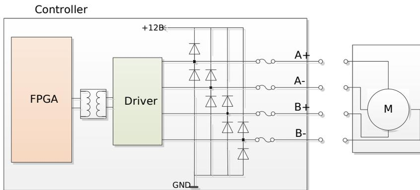
Picture 10 Connection of throttle step motor
