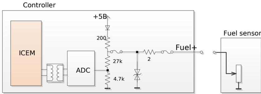
Picture 11 Connection of fuel level sensor
